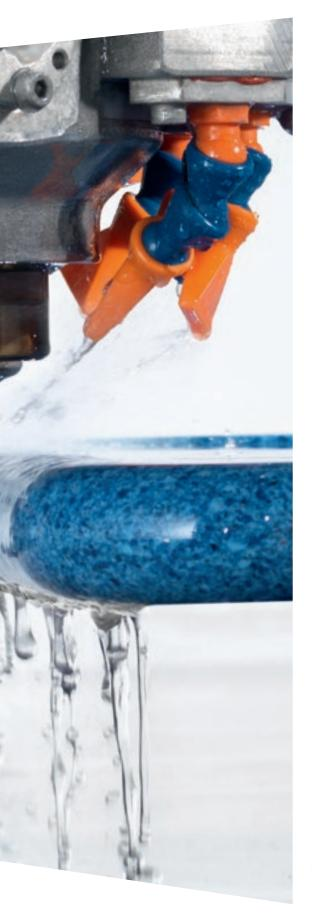
Over 200 of the most widely available profiles in the Diamut catalogue, with the option to creating new ones on request. These are the figures in the Diamut range of profile grinding wheels, available in a whole host of versions starting with a 20 mm diameter, across two different product lines; the KPL and the HYS lines.
