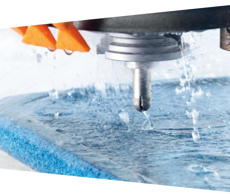
Diamut's range of tools for draining includes shaped milling cutters and scoring wheels for machines equipped with dedicated incision aggregates.
